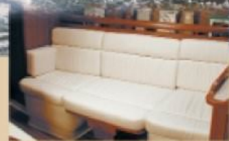
The game table to port stows to become a full length settee or berth.
